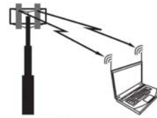
Multilayer transmission ("SU-MIMO") for higher data rates in a given bandwidth
